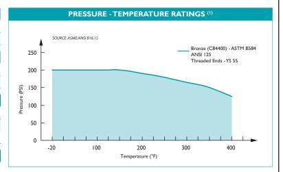
1. The pressure-temperature ratings given are ONLY for the YS 55-BZ (Threaded) per ASME B16.15. The internal working pressure rating for a solder joint strainer is dependent, not only on the strainer, but also on the composition of the solder used for the joint. The working pressure ratings shown for model YS 56-BZ (Solder) are representative of using an alloy Sb5 95-5 tin-antimony solder. For other solder joints, please consult factory.
