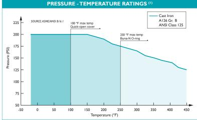
This chart displays the pressure-temperature ratings for the strainer's body material per ANSI B16.1. Max temperature limits have been added for Quick-Open cover and Buna-N O-ring.
