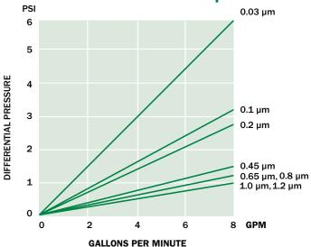
This chart represents the typical water flow per 10" cartridge length. Cartridges are tested in water at ambient temperature. Data may be extrapolated for multiple lengths, but as flow rate increases,  $\Delta P$  of the housing becomes more apparent.
